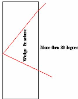
Figure 38. Wedge fracture with obliquity
